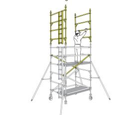
Add two more diagonal braces between the 5th and 7th rungs. If finishing at this height (4.2m platform) reposition the fixed deck to the 8th rung on the tower. Fit a trapdoor deck alongside it, with the hinges towards the outside of the tower, and the trapdoor next to the ladder. Add a single diagonal between the 7th and 9th rungs as shown. Climb up the ladder, and from the protected trapdoor position, fit the guardrails on the 9th and 10th rungs, in that order, on both sides of the tower.
